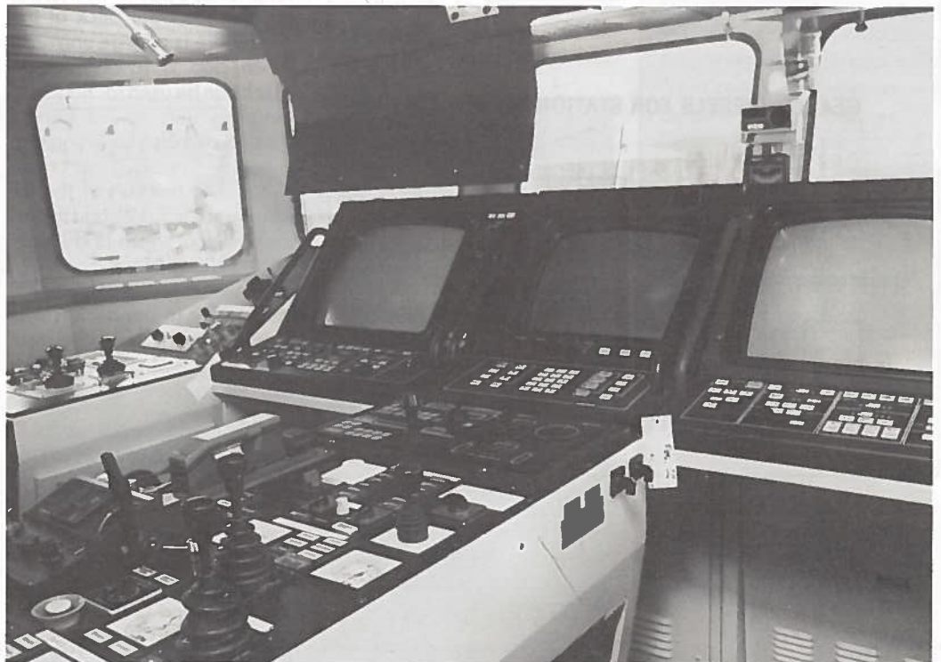
Control panels for dynamic positioning and integrated navigation computer.
